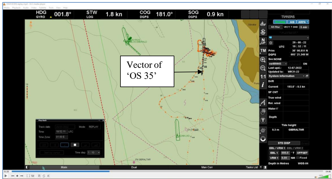
Figure 20 'OS 35' ECDIS display showing the vector with SOG and COG
